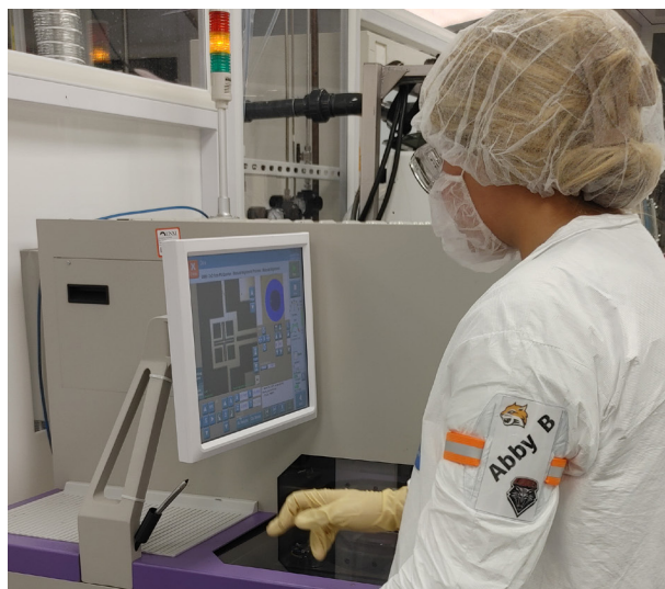
A community college student aligns a wafer to ensure proper alignment prior to dicing the micropressure sensors into individual chips during a week-long learning experience in the University of New Mexico's MTTC cleanroom.
