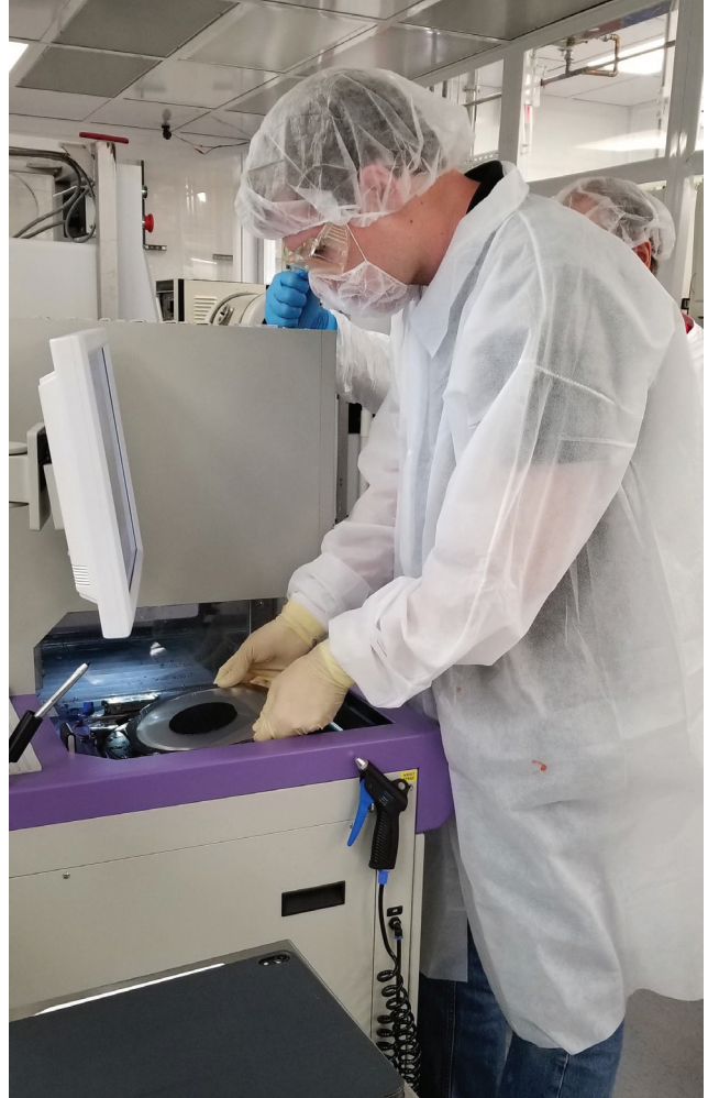
A community college student prepares a silicon wafer for dicing and packaging in the MTTC cleanroom at the University of New Mexico.
