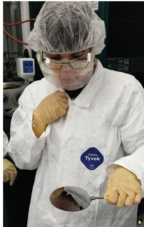
A community college student holds a wafer after sputter deposition of a thin 200nm layer of metal. The wafer will then go through a lift-off process to reveal the final circuit design.
