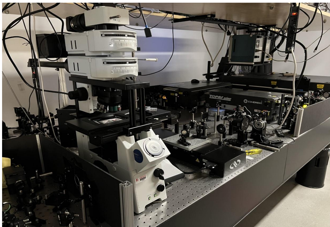
(A) Femtosecond Laser setup at CSUN. (B) Diagram of Femtosecond Transient Absorption Spectroscopy
